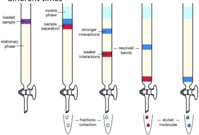
Components of the sample are separated within the column
