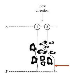
As solute molecules travel through the column, some arrive at the end sooner then others simply due to the different path traveled around the support particles in the column that result in different travel distances.
