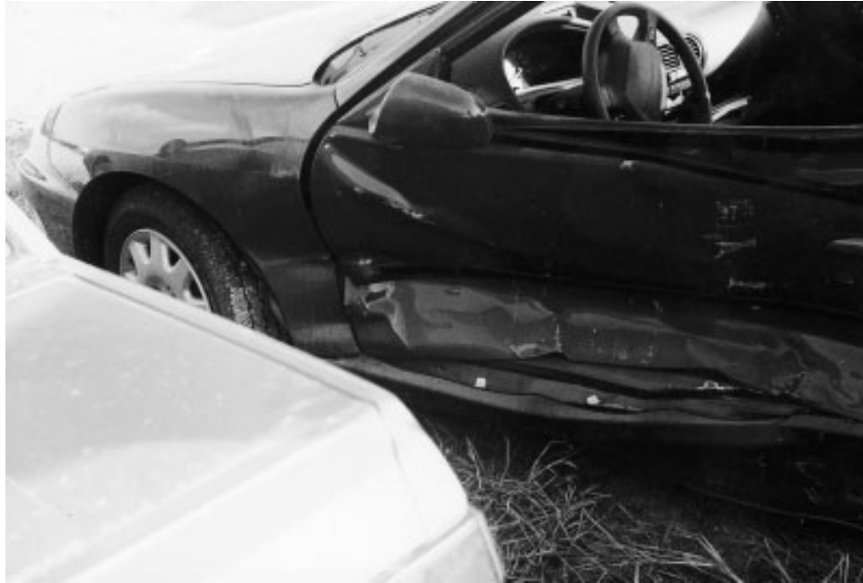
Plate 15.1 Side impact. Note bumper imprint in crush damage along door.
