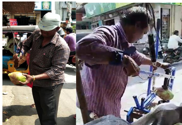
Fig. 8 Tender coconut punching with (a) Conventional method and (b) Coconut punch cum splitter.
