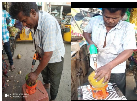
Fig. 10 Tender coconut punching with (a) Tender coco punching tool and (b) Tender coco drill machine.
