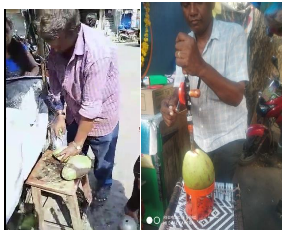
Fig. 9 Tender coconut punching with (a) Tender coconut opener and (b) Manual tender coco opener.
