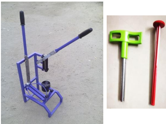
Fig. 1(a)coconut punch and splitter, (b)tender coconut opener
