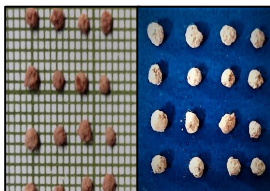
Fig. 1 (b) Harvested crystals of cobalt oxalate
