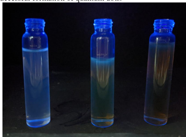
Figure 5: Pure CQD, Succinic acid doped CQD and Cobalt doped CQD under UV light
