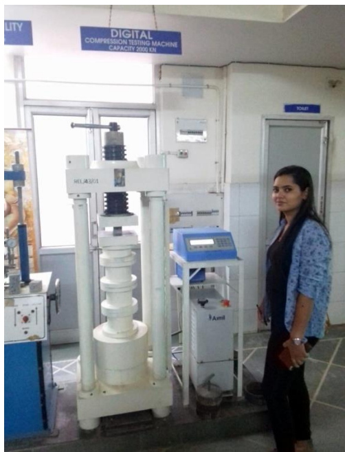
Figure 5: Compressive strength test by the digital compression testing machine.
